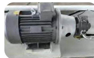
Oil pump motor
